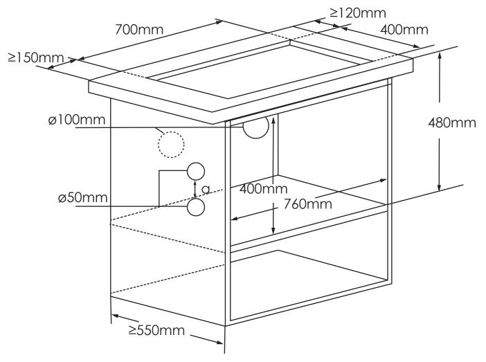
a: The distance between the holes should be >200mm.
