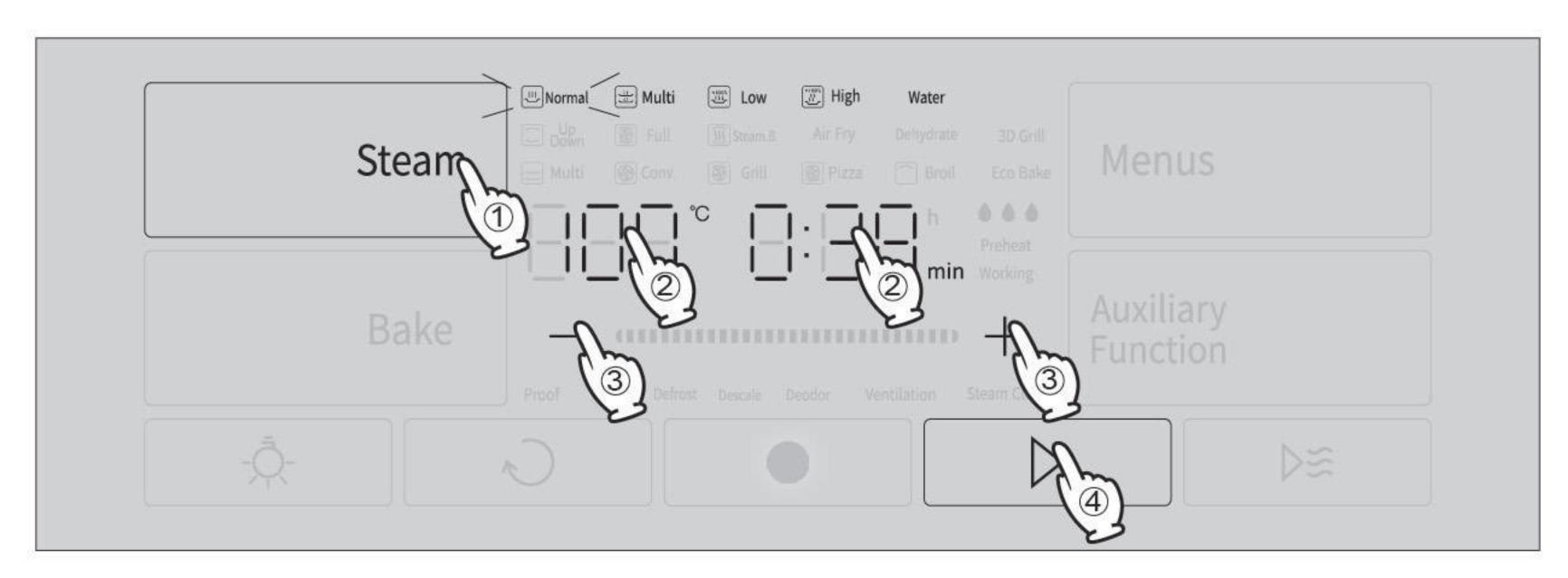
2. **Preheating.** The Built-in-combi oven starts to preheat and displays the current real-time temperature.
