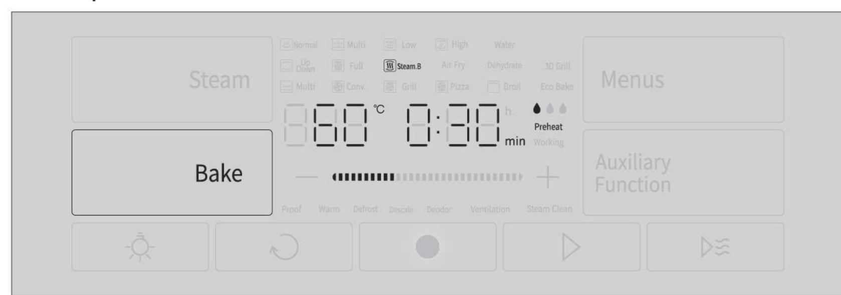
4. **Working.** When the set temperature is reached, the built in combi oven starts cooking and the countdown starts.
