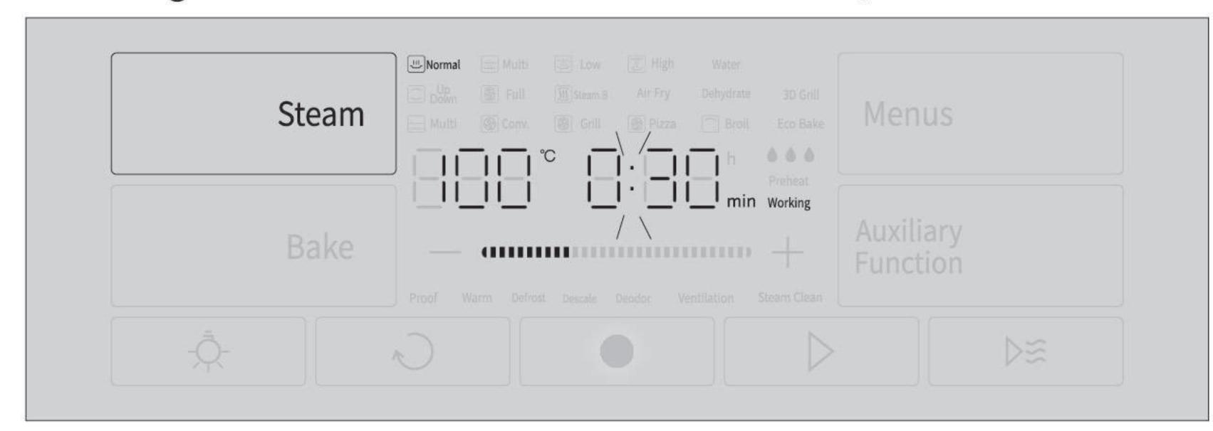
4. **Cooking finished.** The countdown reaches zero, the work is completed, with ten buzzers given.
