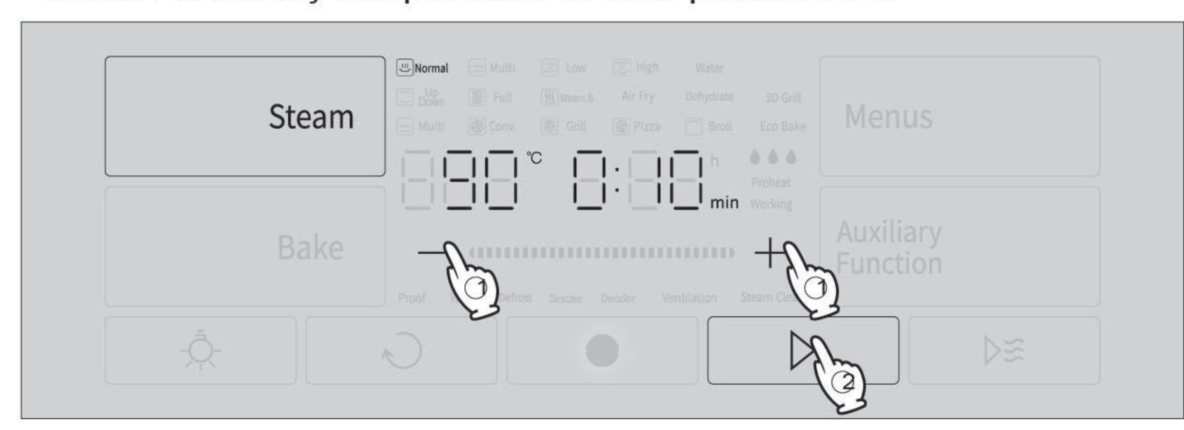
2. Press the button to confirm the modification and continue working.
