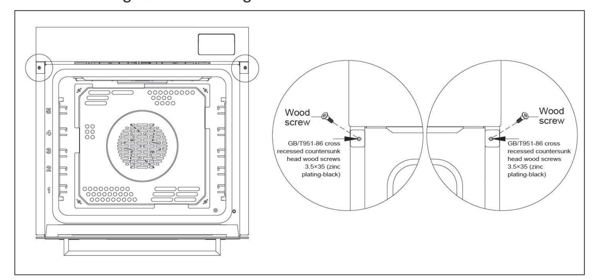
Note: The minimum spacing between each part of appliance and its surrounding structure is 10mm.
