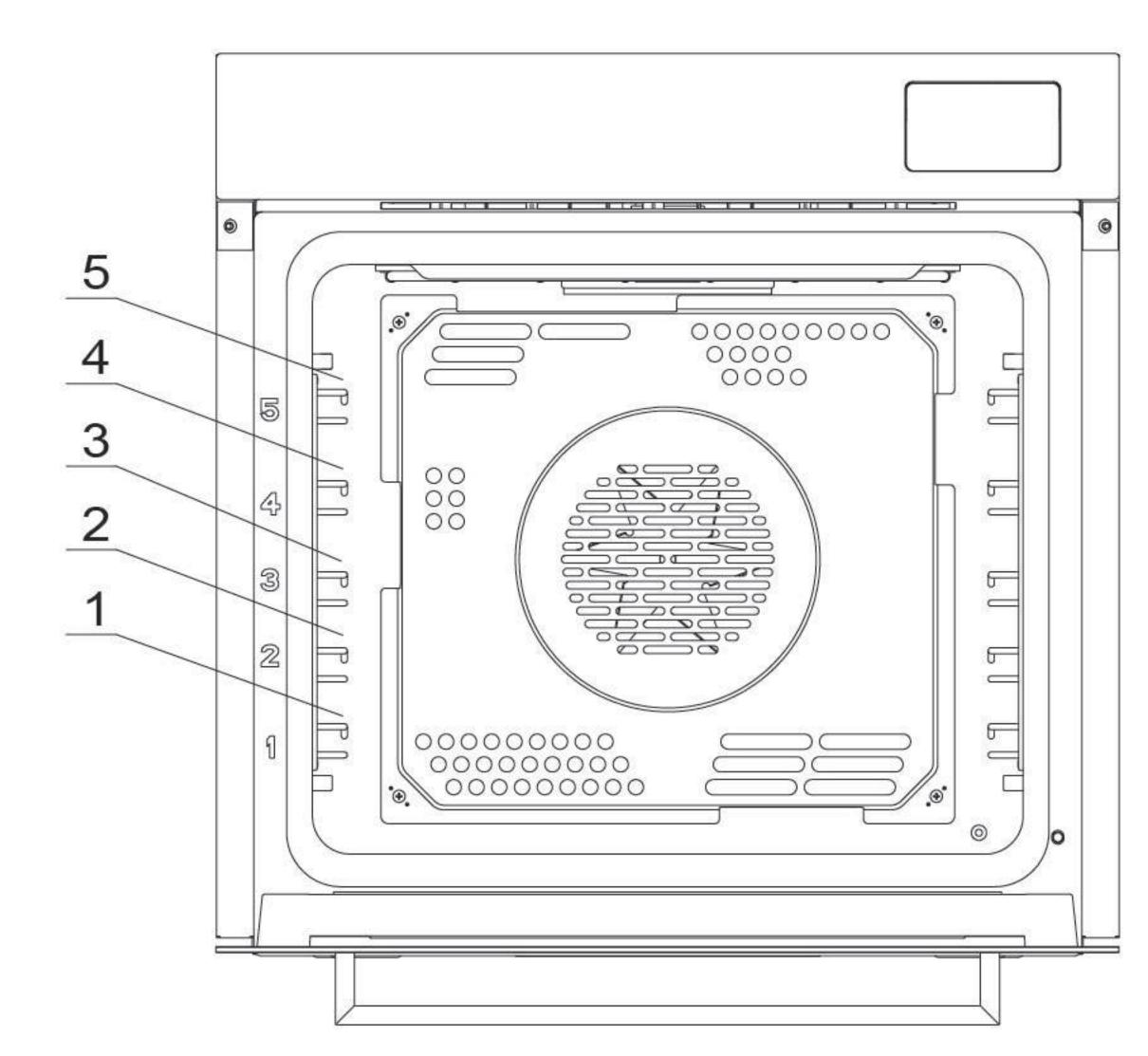
For cooking, 3 layers are recommended. It is recommended to place an oil drip pan on the first layer.
