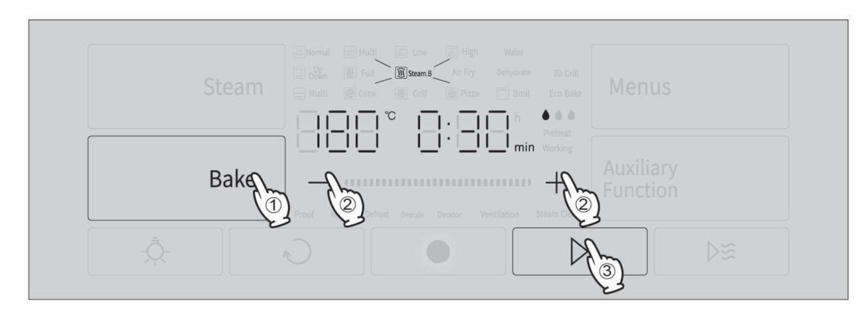
2. Select the gear. Press the water droplet icon to select the desired humidification gear, and click the ▷ button to confirm. The number of water droplet icons in the humidification gear corresponds to low humidity, medium humidity, and high humidity, respectively.
