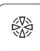
Press &, the button will light up, with "AU" displayed on the screen, After running at maximum airflow for 60 seconds, the range hood, the range hood has entered the "Auto" mode;
